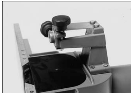
Install cutter guard carrier on the fence. Use 4 each - hexagon head screw M 6x25 - hex. nut M 6 self-locking
